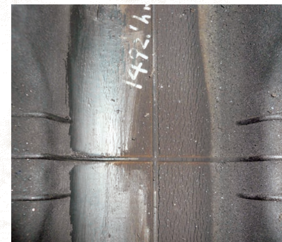
Small ozone cracks
