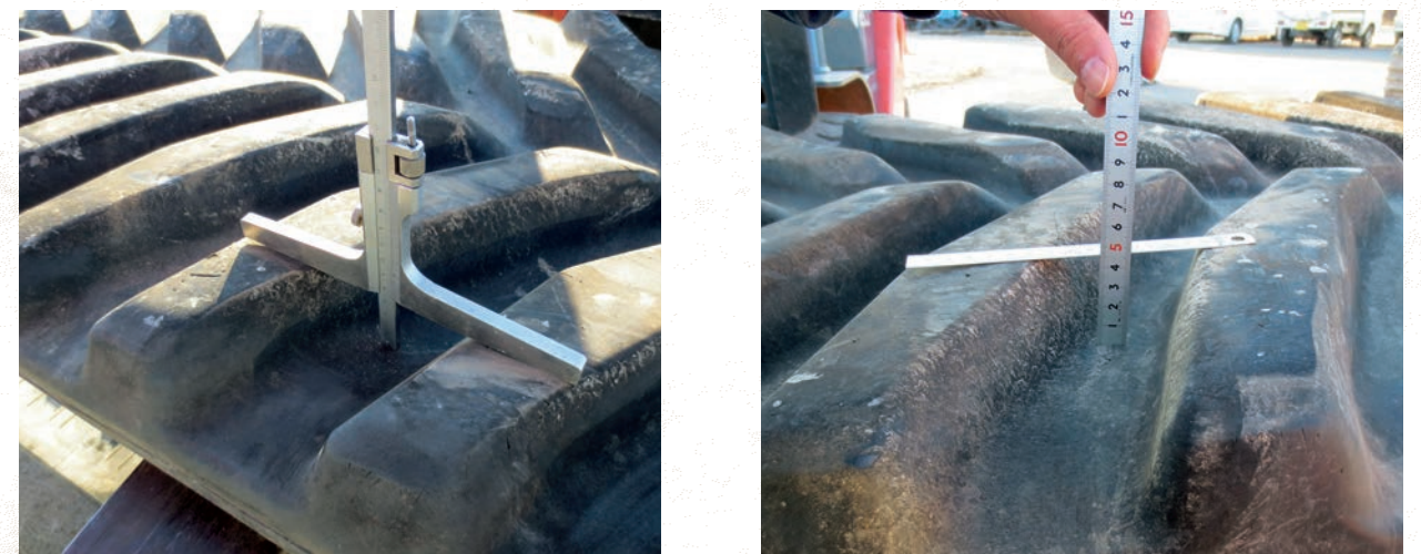
Fig. 1. How to measure the tread depth
