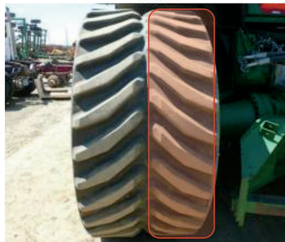
Fig. 1. Accelerated machine side tread wear
