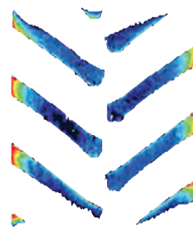
IF CFO RADIAL IF1250/50R32CFO Deep Tread 23° 34100 lbs. @ 23 psi
