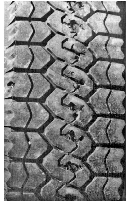
Example of Dyno Damage
